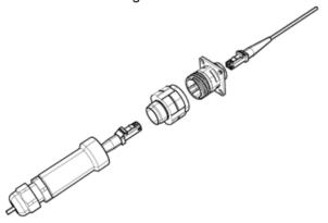
This metallic plug is connected into a receptacle, using a Tri Start Thread coupling mechanism (MIL-DTL-38999 series III type) with an anti-decoupling device for high vibrations.
